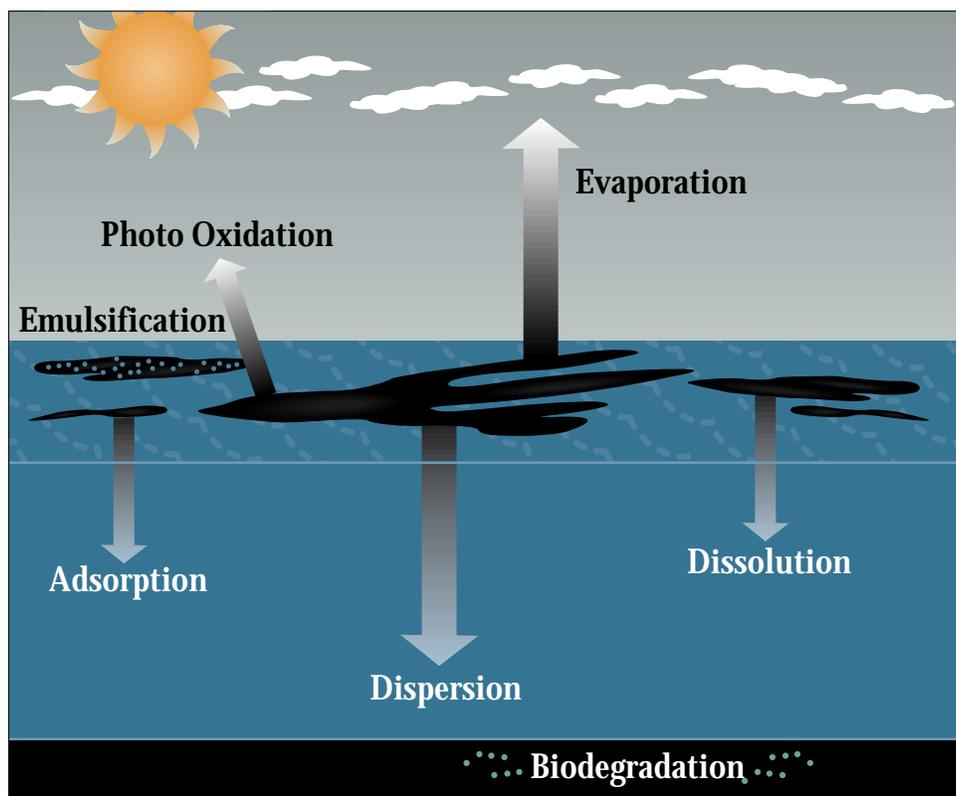
**This figure shows the major weathering processes affecting fuel oil spills. Even at high wind speeds, usually over 70% of a Fuel Oil No. 6 will persist as floating or beached oil for a week or longer.**
